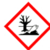
Dangerous for Environment
